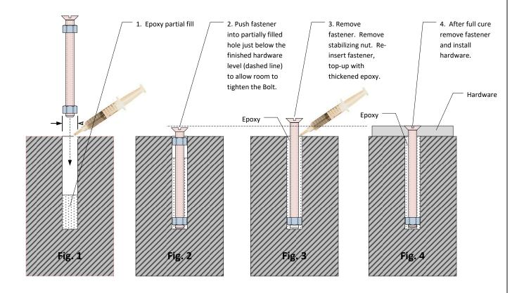
Fig. 1. Drill oversize holes using the hardware to be mounted or a template. Always "dry fit" the hardware and fastener; then apply wax or a mold release such as Evercoat™ to the bolt. Partially fill the hole with thickened epoxy.
