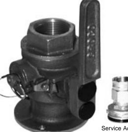
the SBV Safety Seacock is connected can be used as a high capacity bilge pump. To utilize this feature, bilge water level must be higher than the top of the Quick Release Plug Port. First, close the seacock, then grasp the pull-ring, turn the QR plug 90-degrees counterclockwise, and pull the plug straight out. The QR plug cannot be removed unless the valve handle is in the closed position. Your engine can now draw water from the flooded bilge and pump it overboard through the exhaust system.
