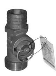
**Maintence:** Remove the Quick Release Plug monthly and lubricate the O-Rings with TFE or Silcon Based grease. Do not use petroleum based lubricant.
