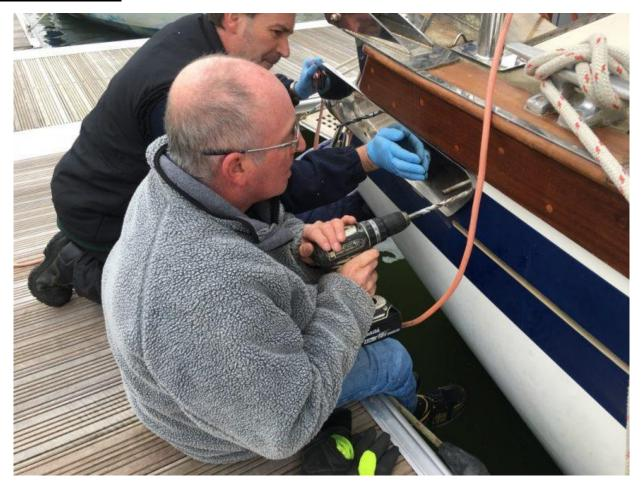
Significant forces are exerted by the drogue under load and anchor points should be substantial and for most fibreglass boats it is likely that both the deck and the cleats will need to be reenforced.
