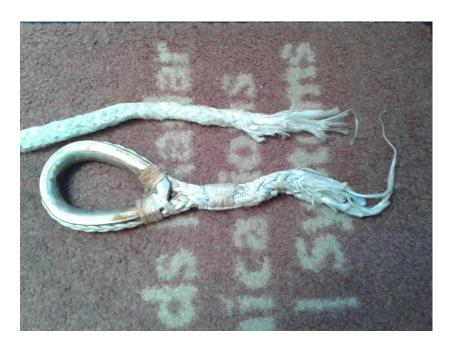
UV degradation is concern so wherever possible the exposed sections of the bridle leg should be protected whenever the bridle is exposed to the sun.
