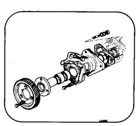
Refit idler gear and time engine. Check backlash which should be 0.004/0.008 in (0.10/0.20 mm).
