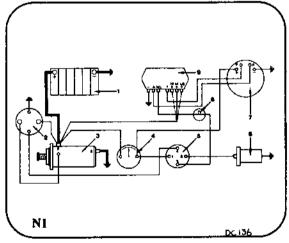
Key to Wiring Diagram incorporating AC5 Alternator.
