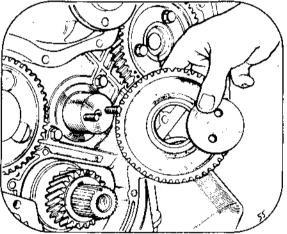
Refit the timing gears ensuring that the timing marks
