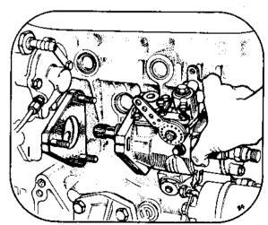
The fuel pump gear will remain in mesh with the idler gear, and will only drop against the inside of the timing case approximately 1/8 in (3,17 mm).
