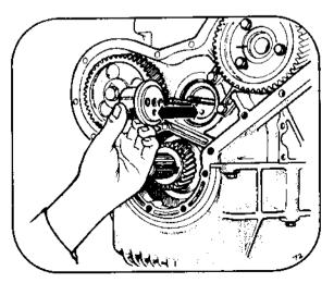
Fit the retaining plate, Fig. F.6, No. 1 and tighten two new self locking nuts to a torque of 19-21 lbf ft (2,6-2,9 kgf m) Fig. F.6. No. 2.
