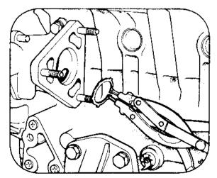
With the gear removed, withdraw the hub. See Fig. F.10.
