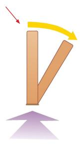
The power in inclined axis vanes diminishes as the vane is pressed over – eventually reducing to zero. This tapering off of their power makes them a lot easier to live with
