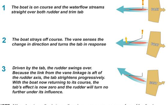
**NOTE:** Although not usually obvious, all modern vane gears use some form of feedback mechanism to tame excessive responses to course changes. Otherwise called 'yaw dampening' – a phrase that explains the objective perfectly.
