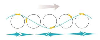
the bottom. Now we should imagine a boat sailing downwind – that's to say from left to right in the diagram. It's blowing hard enough for the boat to sail faster than the wave train. Let's examine what may happen step by step
