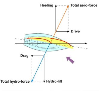
The relationship between these forces determines 'helm balance' – whether good or bad. Now look at the illustration on the right – the same boat side-on, with the centres of drive and resistance marked on the sails and hull respectively. It's easy to see how the boat will heel but, since the two forces are vertically aligned, there's no tendency to turn, either to windward or leeward. The boat is said to be perfectly 'balanced', offering a very easy life for both human and mechanical helms.
